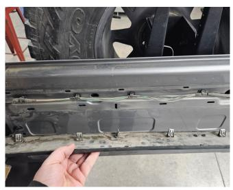
Cut out the alignment locations on the template, and then care carefully align and attach the drill template to the tailgate, using the three clip locations as your alignment guide
