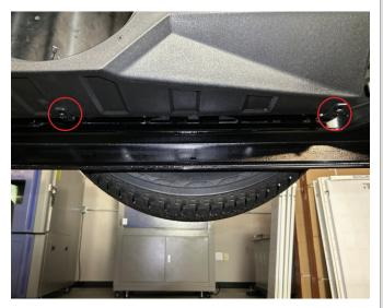
Loosely install (2) M6 x 60mm Hex bolts with 10mm socket.
