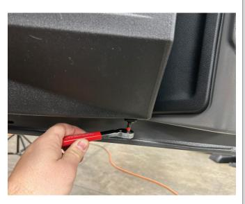
Remove (4) T20 Torx screws holding the subwoofer in the enclosure. Then disconnect the wiring from the subwoofer.
