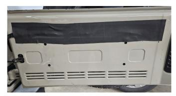
Hold the empty enclosure up to the tailgate to align the four holes in the enclosure to the threaded insert locations.
