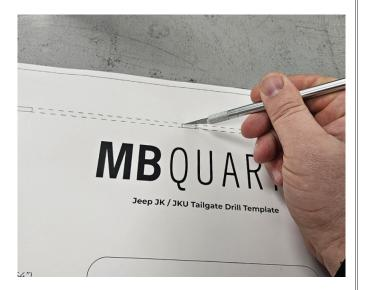
**NOTE:** (On the early versions of this template it is best to line up the top of the 3-template alignment holes with the bottom of the panels clip locations. This is done to land your drill points along the center of the brace inside of the tailgate. These braces are indicated by the small spot welds on the tailgate indicated in blue below.)
