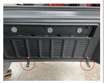
• Loosely install two M6 x 16mm Torx screws with a T40 Torx driver.
