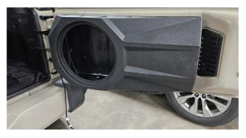
Loosely install the (4) M6x40mm Hex Bolts through the enclosure into the threaded inserts.
