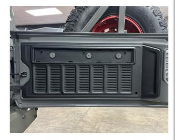
Install two L brackets, 45mm spacers, and M6 x 60mm flathead screws in the bottom two holes of the tailgate panel with a 4mm Allen wrench.
