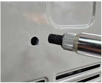
To remove the tool from the threaded insert simply turn the knob at the rear of the tool, to release the threads from within the threaded insert. The threaded insert should remain securely into the hole and not have any play.
