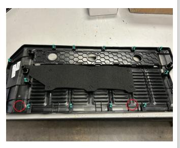
• Install the tailgate panel back into the vehicle by snapping into location.
