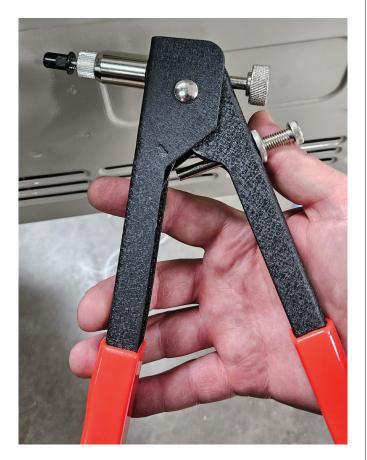
Place the threaded insert into the previously drilled 9mm or 23/64" hole and squeeze the handle until the threaded insert is completely compressed.
