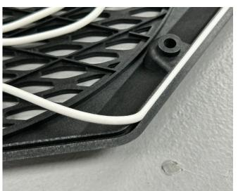
Using panel tool - carefully remove upper tailgate trim panel
