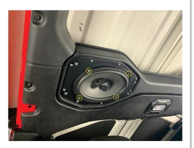
• Mount the new soundbar grill for the 6x9 with the OEM 5mm bolts
