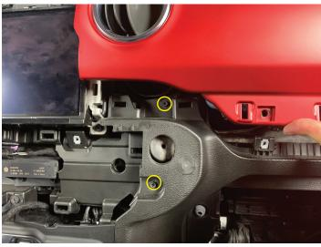
• Remove (2) Phillips screws, disconnect wiring and remove speaker from vehicle
