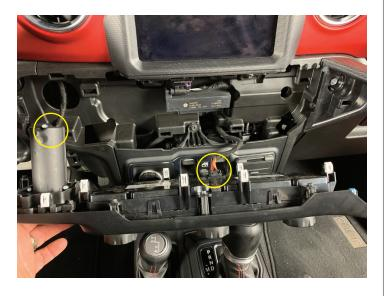
• Remove (2) Phillips screws securing the radio trim panel, then unclip and remove
