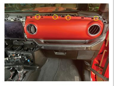
• Unclip and remove the panel on the side of the dash
