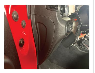
• Remove (5) Phillips screws that are exposed
