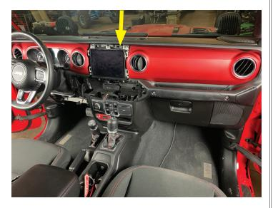
Clip the radio shroud into place and install (2) Phillips screws
