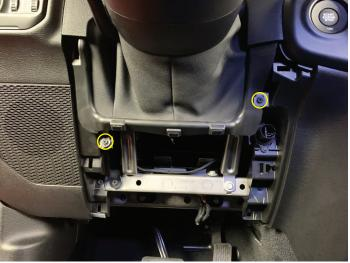
• Unclip, unplug, and remove the climate control panel
