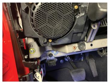
• Remove (3) Phillips screws securing the speaker enclosure
