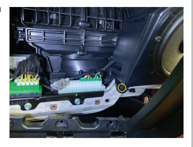
• Install new speaker enclosure and secure with (3) Phillips screws
