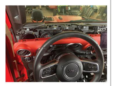
• Install (4) Phillips screws on the driver side securing instrument panel shroud
