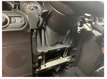
• Install (2) Phillips screws on shroud
