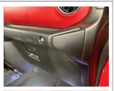
• Install (5) Phillips screws on the side of dash
