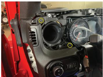
• Install (2) Phillips screws on the top of the left dash
