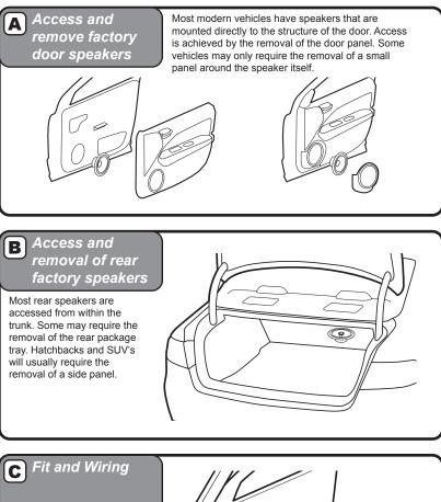
Once the factory speakers are removed, check the fit and determine if there is enough depth clearance for the new speaker. A good way to do this is to roll the window down and back up while holding the speaker in place. If you decide to run wires, make sure to use factory harness boots and grommets where ever possible.
