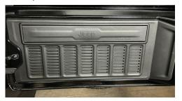
• Using a panel tool carefully unclip the tailgate panel and remove.
