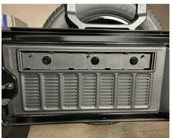
• With the tailgate panel laying face down, drill two 9/16" holes at the dimples at the bottom of the panel.
