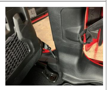
• Unclip the b-pillar sill panel.
