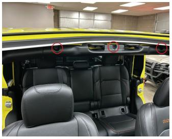
• Carefully remove dome light. Try to use a long flat head screwdriver to depress the clips on either side of the metal clips.
