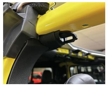
• Pass the dome light connector through the dome light hole on the middle ROPs cover. Then clip the middle ROPs cover to the soundbar.
