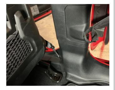
Install passenger side corner panel by clipping back into the vehicle. Then install the fir tree clip. Repeat process on driver side.
