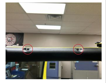
• Install two T25 Torx screws on passenger side front ROPs panel. Repeat last two steps on driver side.
