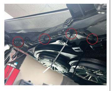
• With wiring secured down the b-pillar, route wiring toward your amplifier and make appropriate wiring connections.
