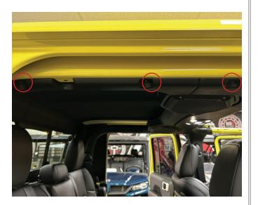
• Remove two T25 Torx from the passenger inside rear ROPs. Then carefully unclip and remove from the vehicle. Repeat the previous two steps on the driver side.
