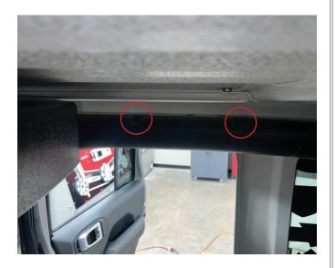
• Install three or four T25 Torx on the passenger side rear ROPs. Repeat the last two steps on the driver side.
