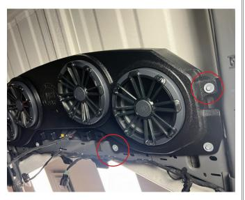
• Route the soundbar wiring along the OEM wiring toward the passenger b-pillar sill panel and then down to the floor. Secure wiring with zip ties.
