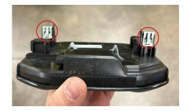
• Carefully unclip the middle ROPs cover from the OEM soundbar and remove from the vehicle
