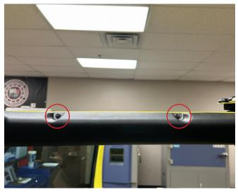
• Remove three or four T25 Torx from the passenger side rear lower ROPs.
