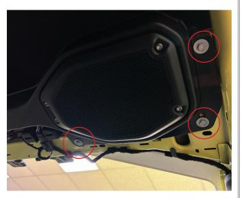
Install the MB Quart Soundbar using the bolts from the previous step.
