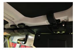
• Remove four T25 Torx from the passenger side front ROPs (Rollover Protection System) and then carefully unclip and remove from vehicle and set aside (Repeat on driver side).
