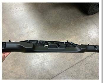
• Using a panel popper, remove the fir tree body clip on the front corner edge on the passenger side ROPs. Then carefully unclip the panel and remove from the vehicle. Repeat process on driver side.
