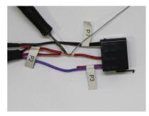
**Step 6.** Once the wires are soldered together, use heat shrink or electrical tape to insolate the wires.
