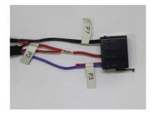
**Step 5.** Solder the wires together.
