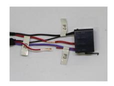
**Step 4.** Once shielding is removed, wrap the red wire from P3 around the exposed area of the red wire from P2.
