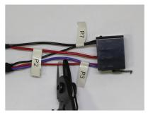
**Step 3.** After cutting the red wire on P3, strip back the plastic shielding on the red wire of P2.
