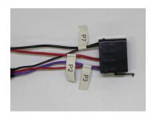
**Step 2.** Cut the red wire while leaving the purple wire connected to the switch.
