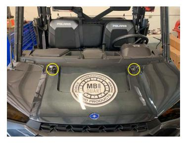
• Remove two push pins from center and pull radio forward
