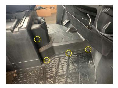
• Remove five push pins from the driver side center console
