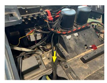
Pass the wiring around any moving parts and down the frame toward the center console and secure in place with zip ties
