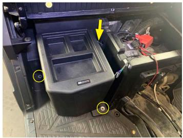
Connect the subwoofer enclosure harness to the subwoofer extension harness
