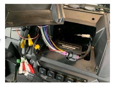
• Install the radio assembly and attach with two push pins
