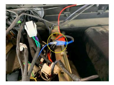
Route the rear speakers and subwoofer extension harness from the middle of the dash out the grommet toward the front of the vehicle
