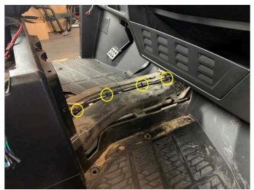
Route subwoofer and rear speaker harness to the passenger side of the battery
