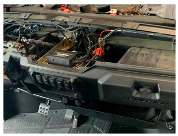
• Remove four push pins from the passenger side center console
