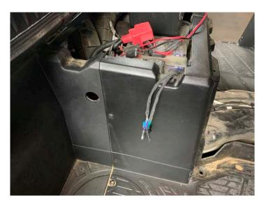
Drill 1.25" hole and pass subwoofer connection through hole and place grommet
