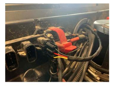
Pass the amplifier power harness from the front of the vehicle into the cab through the grommet
