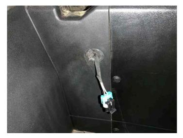
If four-seat vehicle, connect extension harness to route rear speaker wires to the back of the vehicle (if installing rear pods jump to that section)
