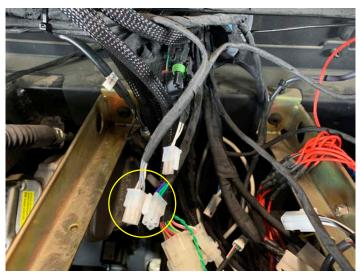
Pass the wires from the grommet to the radiator cap opening if other wire present zip tie along
