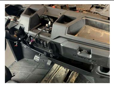
• Install three push pins on driver side of dash
