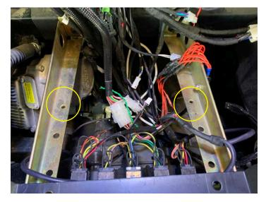
Raise the plate and install two 10-32 x ¾" bolt and washer into amplifier plate
