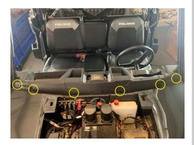
• Lift up on the dash and remove from vehicle
