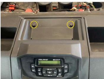
Remove two push pins from instrument cluster. Remove and disconnect connector on back
