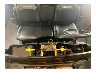
Reaching from the top of the driver side of the dash, pass the white wires through the top of the pocket and insert the grommet
