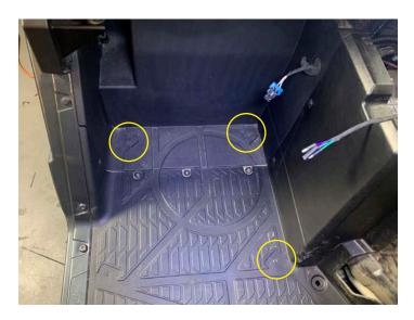
Place subwoofer enclosure under passenger seat and secure with three high-low T25 Torx screws and washers
