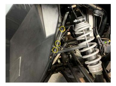
Run along air intake securing with zip ties to the power bus bar harness
