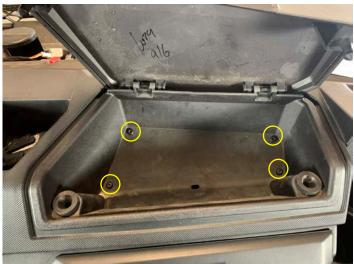
• Install six push pins on the front side of the dash
