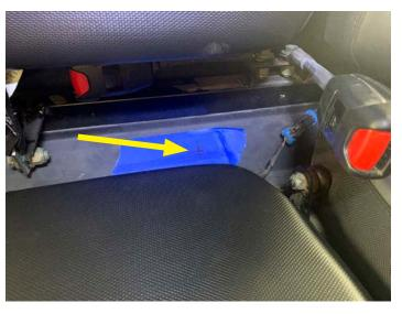
• Drill 1/2" hole, then pass rear speaker wire from battery compartment out to inside of passenger cabin
