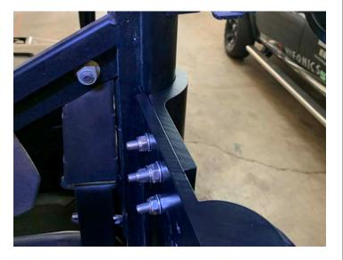
Install pods with four M6 cap head bolts using a 5mm Allen wrench, then connect wiring
