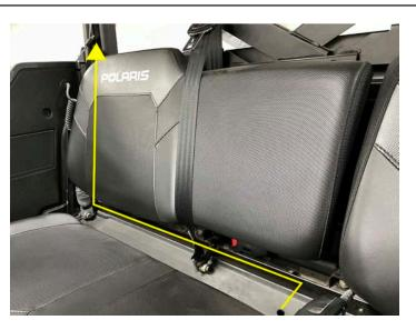
• Place one adhesive channel on driver side under seat on frame
