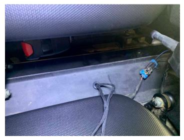
• Place two adhesive channels on passenger side under the seat on the metal frame
