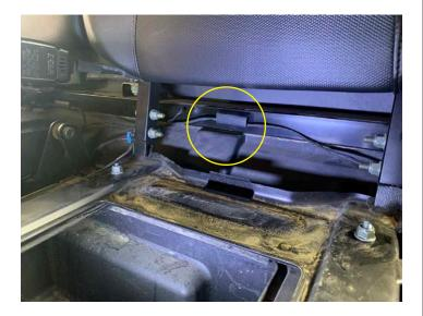
Route driver side green speakers wire-in channels toward driver door then route upward toward the ROPS (avoiding any moving objects), secure, and attach one adhesive channel on ROPS
