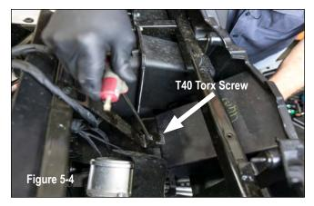
Set aside OEM dash clip for source unit mounting later in the installation if you are installing an MB Quart MBQR-RAD-2 or simply reinstalling the pocket.
