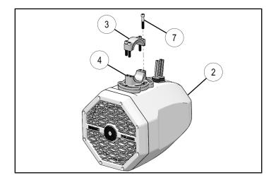
Place bushings (a) into upper and lower clamps (a)
