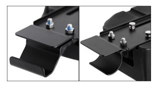
Install sound bar in vehicle adjusting top brackets so it is sitting on the ROPS. Then with which ever clamp your vehicle needs attach it to the flat bracket with a 5/16" bolt, lock washer and nut.
