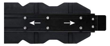
When the bolts are loosened, the bracket can slide to accommodate a variety of roll cages whose inside roll bar dimension is between 37.25" - 58.25" for the MBQOH-33-1, 44.25" - 61.25" for the MBQOH-41-1, and 49.25" - 66.25" for the MBQOH-46-1. Once the proper width has been established, these bolts should be retightened to a torque specification of 40-45 inch/lbs.
