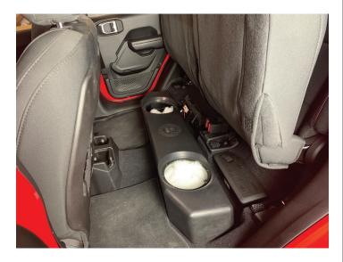
Connect the subwoofer speaker wires to the subwoofer and repeat the process for other subwoofer
