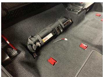
Connect subwoofer enclosure wiring to subwoofer extension harness.
