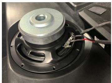
Secure the subwoofer to the enclosure with (8) High-Low screws using a T-20 Torx bit
