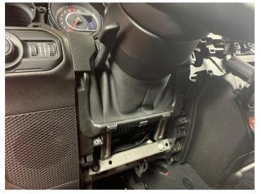
• Install (2) Phillips screws on shroud
