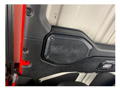
Remove and disconnect (4) T30 Torx screws from the port and (5) T20 Torx screws from both speakers
