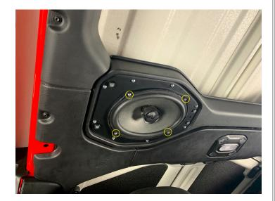
• Mount the new soundbar grill for the 6x9 with the OEM 5mm bolts
