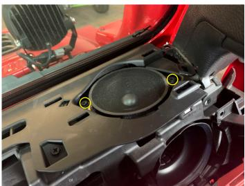
• Connect the factory wires to the speaker
