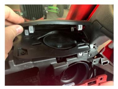
Remove (2) Phillips screws, disconnect wiring and remove speaker from vehicle
