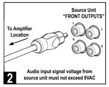
Route left/right preamp-level RCA audio cables and remote turn-on wire from source unit preamp outputs to the amplifier's installation location.
