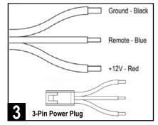
Route power+ground amplifier wiring to the amplifier's installation location. Including remote turn-on, connect wires to 3-pin power plug as shown.
