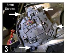
If the vehicle has the Smart-Lok differential control module, attach to the underside of the new dash panel with the original four 8mm screws.
