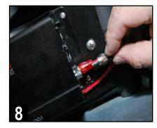
Connect the RCA audio cable fron source unit to left and right channel amplifier inputs. Be sure to double check left is left and right is right (channel).
