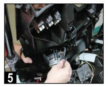
Connect driver side speaker to your installed speaker wire. Crimp connectors are needed to mate with speaker terminals.
