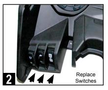
Replace switches in the same locations within the new MB Quart driver's side dash panel by simply pushing each into its mounting opening.
