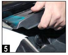
Remove top center plastic cover above dash pocket by pushing up on the front pocket edge above the lighter socket, then pulling toward you.
