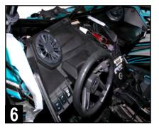
Set panel temporarily in place without attaching any hardware or clips. Do not yet plug in switches in case amplifier adjustments are needed.
