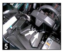
Drop steering wheel position to access two T-30 gauge cluster screws. Cluster removal helps removal of the panel and access for amplifier installation.
