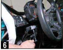
Remove two T-30 screws holding the gauge cluster with a 10mm socket (below) and T-30 driver (above). Set gauge cluster aside when done.
