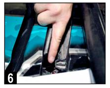
Next, remove two additional T-30 screws located beneath the forward edge of the top center plastic cover location, just forward of fuse box.
