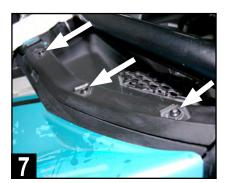
Remove three T-30 screws from the top edge of the driver's side dash where the hood line meets the dash as indicated.
