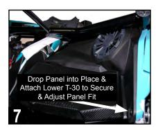
Next, drop the speaker edge of panel into place\*. Attach lowest T-30 screw into place to allow check of final panel fit and to ensure all clip holes align.
