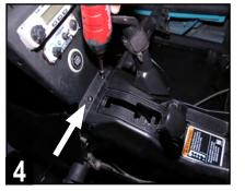
Move gear selector all the way back (away from the dash). Remove two T-30 screws from the area just forward of the gear selector when in park.
