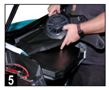
Begin to set passenger side speaker panel in place by loading the edge nearest the center with the clip retainers into position as shown.
