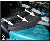
Remove three T-30 screws from the top edge of the passenger's side dash where the hood line meets the dash as indicated.
