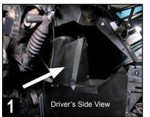
Prepare to remove forward inner cover of the center console. Note - some modified vehicles may have aftermarket console electronics present.
