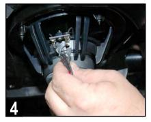
Connect passenger side speaker to your installed speaker wire. Crimp connectors are needed to mate with speaker terminals.
