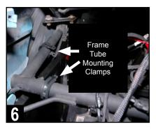
Route power, speaker wiring and RCA audio cables to amp mounting location (near frame tubes). Place mounting clamps in initial locations as shown.
