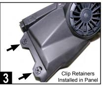
Replace these mounting clip retainers and washers in the same locations of both MB Quart speaker panels in your Can-Am X3 kit. It's a direct fit.
