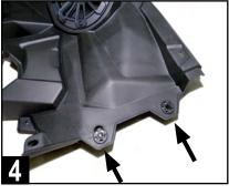
Ensure the clip retainers and washers from the original dash panel have been reinstalled correctly before proceeding.
