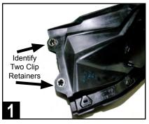
Locate the factory front left and right speaker panels and identify two mounting clip retainers and washers that need to be removed on each.
