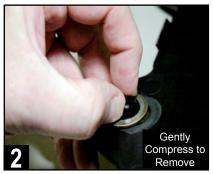
From bottom side, gently remove mounting clip retainers as indicated. This can be done with your fingers. Do this for both passenger and driver side.
