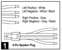
Route speaker wiring from each front speaker location to the amplifier's installation location. Connect wires to 4-pin speaker plug as shown.
