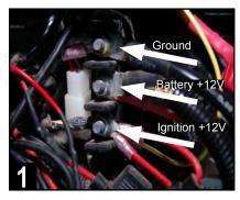
Identify bus bar in passenger side center console. Top is chassis ground, middle is constant +12v power (battery) and bottom is +12v ignition.
