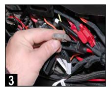
Remove the fuse from the main fuse holder you've installed so the power wiring is not live while routing through the vehicle.
