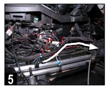
Continue routing your wiring forward along the passenger side console as indicated by the arrow and zip tie to factory wiring.
