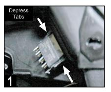
Remove switches on lower left of original driver's side dash panel by depressing the tabs on the top and bottom of the back of switch.
