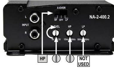
• HP - Rotate control to halfway from 15 Hz (pointing up). This is approximately 80Hz\*.
