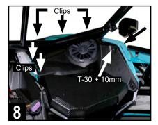
Secure the front speaker panel by reinstalling all the remaining clips and hardware in the same locations removed during the disassembly process.
