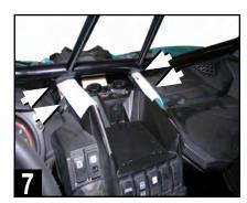
Identify four visible push pin clips on the outer edges of the center pocket. These secure the flanges of the left and right side dash speaker panels.
