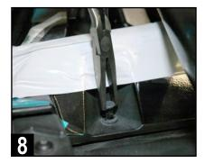
Gently remove the four visible push pin clips with a panel removal tool or special panel clip pliers (not needle nose) as shown.
