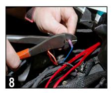
Crimp or solder connections to the source unit's power wiring connector. Extend the source unit's remote turn-on wire to the amplifier mounting area.
