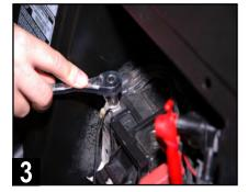
Repeat seat removal on front passenger's side (and rear seats - if present). Once passenger seat near battery is removed, disconnect (black) negative battery cable by removing a 10mm bolt and set the negative cable aside.
