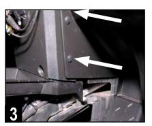
Finally, remove two push pins on passenger's side of cover panel.
