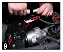
Connect the 4-pin speaker and 3-pin power wire harness connectors as shown. Zip tie wiring to void any moving parts, moisture or heat sources.
