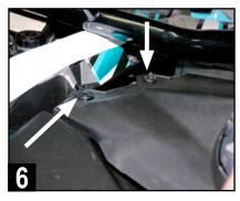
Pull center edge of panel up to align clips with the respective dash receiver holes. This is a crucial step to facilitate the correct overall panel fit.
