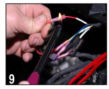
Use high quality electrical tape or a lighter/heat gun to heat shrink any connections. This ensures no moisture will penetrate the wiring
