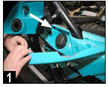
Remove gas filler access door on passenger side. Note above the grommet for the retainer clip, there is a 10mm nut attaching a mounting screw.
