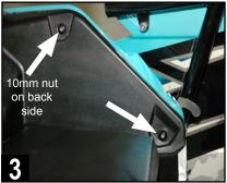
Remove the remaining two T-30 screws on the side edge of the panel. The top screw requires the 10mm nut loosened with a 10mm socket.
