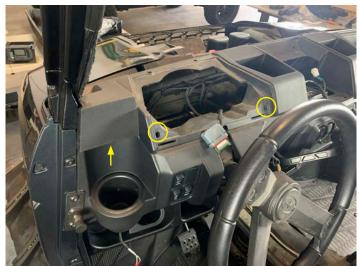
Connect harness and place the instrument panel in location, then insert two push pins
