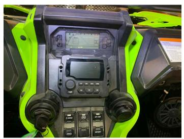
Install four M4 cap head bolts through the face of the radio and dash into the u-bracket and tighten
