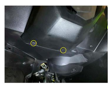
• Remove the bottom steering wheel cover
