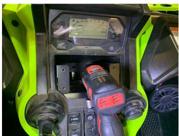
Install two 5mm allen bolts through the bracket and pocket and install a flat washer and lock nut (you may need to ask a friend for help or can reach on both sides of the dash to tighten)
