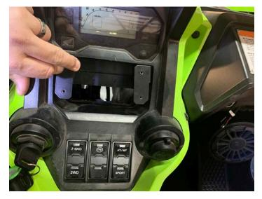
Drill two ¼" holes using the u-bracket as a guide in the back of the pocket
